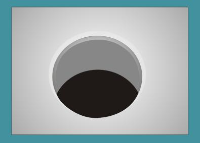
Providing & Applying PU Base Flexible Water Proofing layer sandwich with Polypropylene double layer membrane over the junction of the drain.
