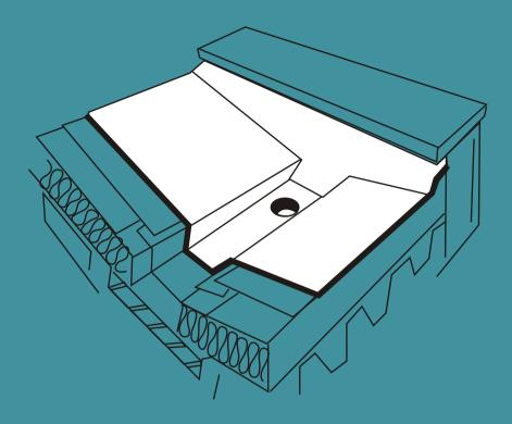
Providing & Applying PU Base Flexible Water Proofing layer sandwich with Polypropylene double layer membrane between the concrete / metal gutter section.
