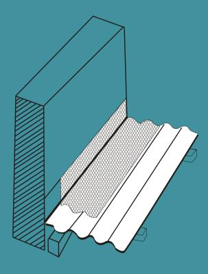
Providing & Applying PU Base Flexible Water Proofing layer sandwich with Polypropylene double layer membrane over the sheet & wall section.
