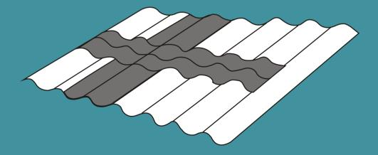
Providing & Applying PU Base Flexible Water Proofing layer sandwich with Polypropylene double layer membrane over the sheet overlaps section.
